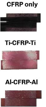
Figure 5 – Failure mode of SLJ's.
